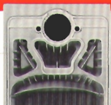
Multi-Finger Surface Finger-like projections in the path of the hot gases extract more heat. Heat Conservor Baffles force gases against fingers and stretch heat travel.
