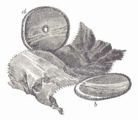
bent outwards. The thickness of the copper along the line of rupture varies from 0.25 to 0.35 of an inch, and the metal appears to have been highly heated at one end
