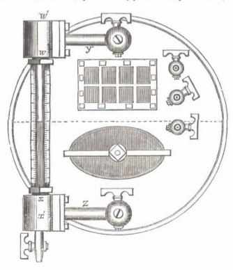
from, the tubes connecting them with the boiler, which are provided with stopcocks: coupling screws might, in practice, be substituted for these conical terminations. To protect the tube, w x, from currents of air, it was surrounded by a second tube, loosely applied. A scale was attached to w x, to indicate the level of the water within the boiler. instrument, its inconvenient length, or position in certain cases, and its
