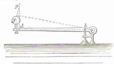
The lever would have a form similar to the annexed. The part ag, which is turned up, may be straight or otherwise. The adjustment should be made so that dc is nearly nine-tenths of ac. g being the centre of gravity of the ball, lever, &c. will lie a little out of the centre of the weight, towards the fulcrum.
