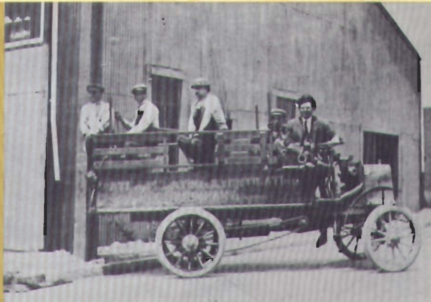
A HEATING EQUIPMENT truck in 1908 with chain drive and no headlights or windshield.
