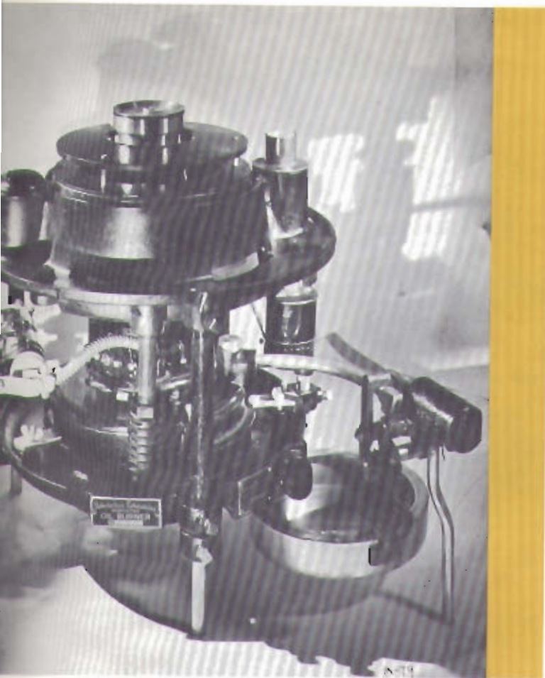
THIS ABC ROTARY burner had a 10,000 rpm direct driven vertical shaft atomizing cup. Trip bucket safety switch at lower right.
