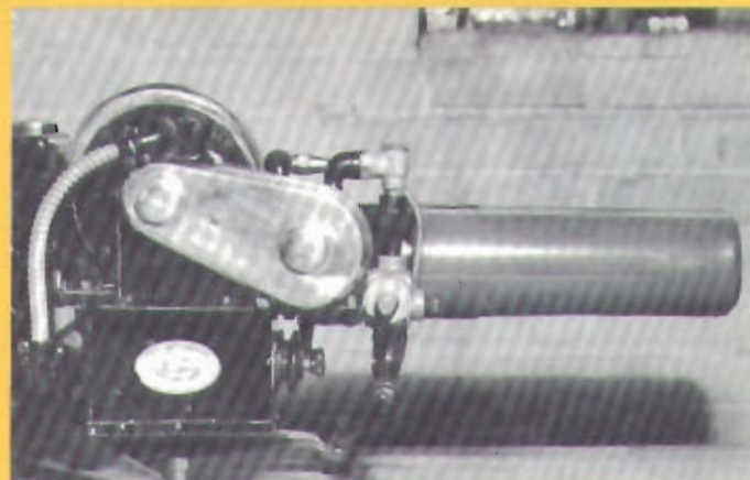
AN EARLY model belt driven Nu-Way with burner mounted control relay and stack-switch in smoke pipe.
