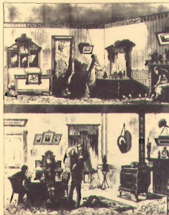
HEATING an upstairs room from stove with air circulation attachment.
