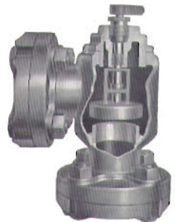
Illustrating interior construction of B & G Angle Flo-Control Valve.
