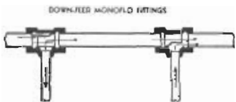
Down-fed radiators must be equipped with a Down-fed Supply Monoflo Fitting and a Down-fed Return Monoflo Fitting.
