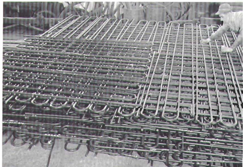
Ground floor piping in office building, showing Rayduct being welded. Rayduct floor coils are also used in heating the second floor of this structure. Right: Pile of prefabricated Rayduct coils ready for shipment to project in Metropolitan area.
