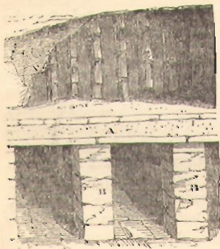
Figure IX. is a section of a portion of one of the hypocausts. B B, the piers; A, the floor of the hot water
