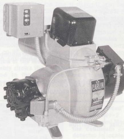
Typical bracket-mounting of primary relay (Honeywell "Protectorelay" R8184 or R8185D) for use with cadmium cell flame detector. Burner illustrated is Model 450FR-2. Bracket accommodates either Honeywell or White-Rodgers controls. The primary control is so mounted that it is well within the over-all width of the burner and back far enough to permit use of the total effective air tube length.
