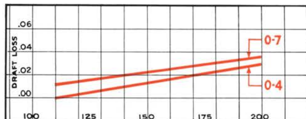
OUTPUT % OF RATED DIRECT CAST IRON RADIATOR LOAD. CURVE BASED ON 12.5% CO 2 .
