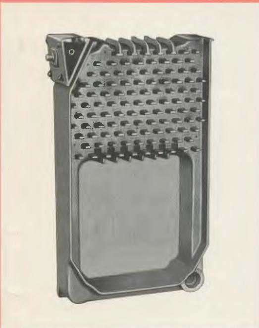
Rugged cast iron sections heat fast, hold heat longer and are rust and corrosion resistant. The patented 'Free-Floating' construction provides independent expansion of each section. A unique V-shaped, rubber-cushioned header allows boiler water to flow unrestricted between sections, equalizing boiler water temperature and assuring peak operating efficiency.
